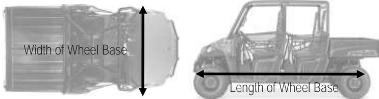
Tow Vehicles vary greatly in overall size. Length and width of wheel base do matter. We have developed the PR90 Series to more effectively cover wheel tracks of large tow vehicles (especially when turning). Tight turns should always be avoided.
