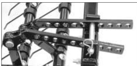
Tine Adjustment System. Easy to choose and set to make the amount of contact desired.
