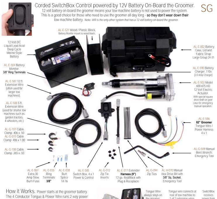
The 4 Conductor Tongue & Power Wire runs 2 way power towards the operator (through whichever extension wire is used) and onto the SwitchBox. From switch 2 way control is returned to the actuator on groomer.
