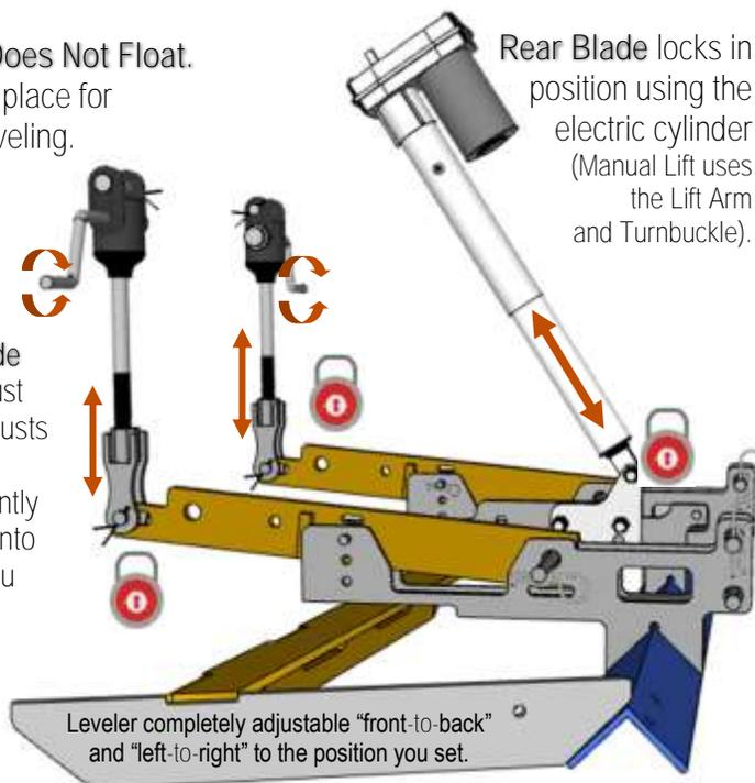
Rear Blade locks in position using the electric cylinder (Manual Lift uses the Lift Arm and Turnbuckle).
