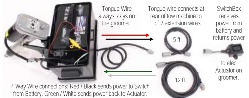
**Advantages:** 12 volt electric system completely on-board the groomer provides all the power needed for lift / lower functions.
