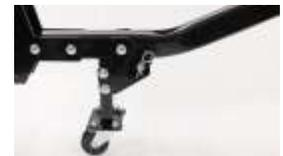
Connects behind hitch on tongue. When groomer unhooked stand keeps end of the tongue off of the ground or floor. When storing the groomer caster wheel allows for easier movement around storage area.
