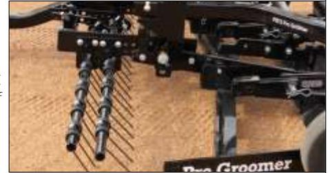
Warning: The Spring Tine Scarifier adds approx. 48 lbs. to the front of the groomer (tongue weight). This adds to the total weight when lifting on the tongue to connect the groomer to a tow machine (or when disconnecting). This is most noticeable for those who have the "WR" electric lift system which includes a heavy 12 volt battery on board. This combination of the Tines and Battery make the tongue quite heavy when lifting.
