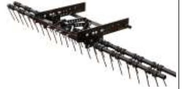
Two rows of staggered spring tines. Each row independently adjustable (without tools) to different angles. Mounts to front of the groomer.
